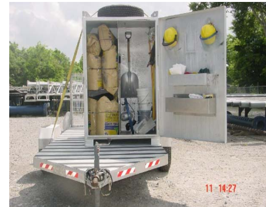
LAND MODEL - OIL SPILL CONTROL LOCKER
