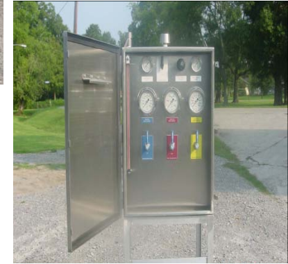
WELL CONTROL PANEL/PRESSURE TEST PUMP
